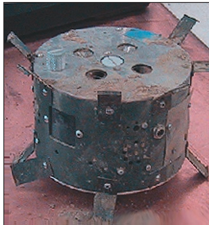
Figure 1. Self-healing minefield node shows wear from a system demonstration including hopping.
