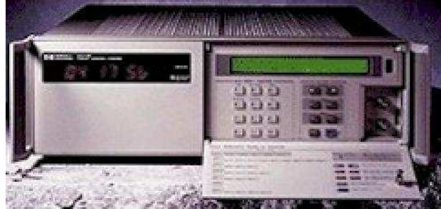
Figure 2.1: left ) The NIST-F1 cesium fountain atomic clock—the most stable in the world since its completion in 1999, developed by Steve Jefferts and Dawn Meekhof at the U.S. National Institute of Standards and Technology. (Photo copyright 1999 Geoffrey Wheeler, used with permission of NIST.) right ) A commercially available cesium clock—the Agilent (formerly Hewlett-Packard) 5071A.
